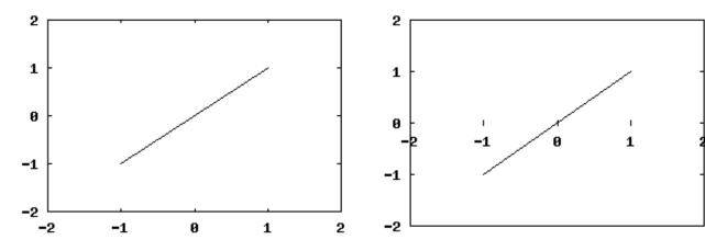
• Mirror tics on opposite axis? "Yes" or "No". If the location of tic marks is set to "border" this parameter determines if they are shown on both the top and bottom or right and left sides of the graph. The "mirror" tic marks are unlabelled.
